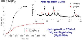
The resulting mixture was converted to  $\alpha$ -MgH<sub>2</sub> by heating in a H<sub>2</sub> medium at 150 °C for 2 h. Analysis of hydride profile parameters indicates that the size of crystallites is <10 nm.
